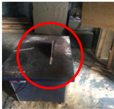
2.车间木工电锯危险部位裸露
